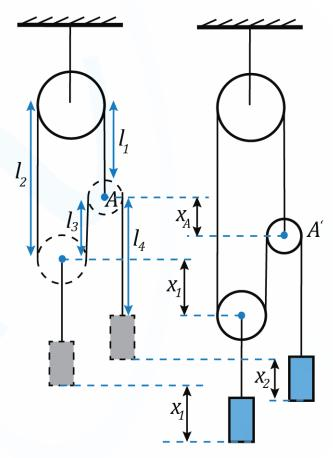
For the case of non-stretchable rope, total length of the string should be constant for any moment of time:
