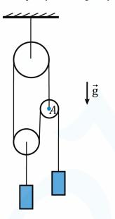
As the rope is weightless, tension force T should be equal in any point of the rope.
