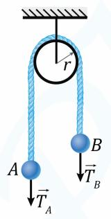
If there is no slippage between the rope and pulley and no friction in the axle of the block, equation of rotational dynamics for the pulley with moment of inertia *I* can be written as
